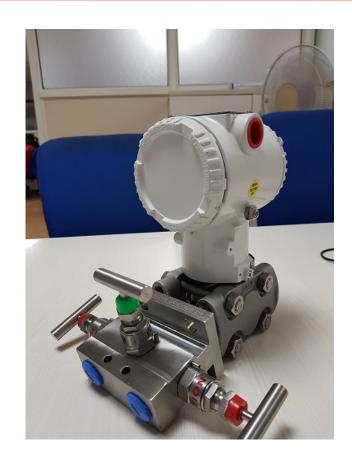
3 WAY T-TYPE (INTEGRAL) MANIFOLD CAN BE DIRECTLY FITTED ON TO THIS DP TX AND THE PROCESS CONNECTION ON MANIFOLD OUTLET IS ½" NPT (F) AS PER PROCESS REQUIREMENT
