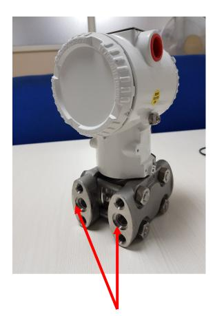
THE STANDARD PROCESS CONNECTION FOR ABB DPT IS 1/2" NPT (F)
