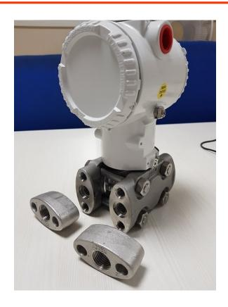
IN CASE YOU NEED ½" PROCESS CONNECTION ON DP TX, ABB WILL PROVIDE ADDITIONAL SS 316 ADAPTOR WHICH WILL GET FITTED ON TX.
