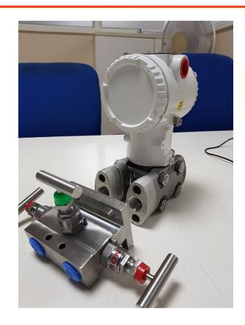
IN THAT CASE YOU CAN'T FIT 3 WAY T TYPE INTEGRAL MANIFOLD ON THIS OVAL FLANGE
