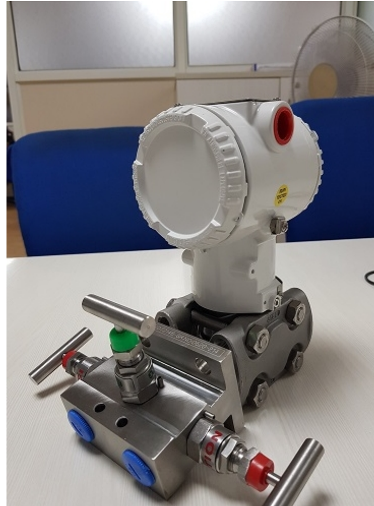
3 WAY T TYPE SS MANIFOLD FITTED ON DP TX
